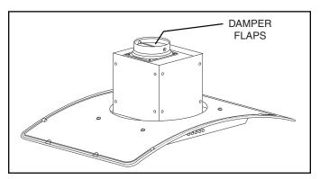
1. Remove the damper flaps from the damper / duct connector and discard flaps.
