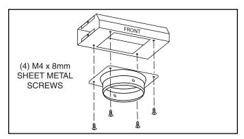
2. Attach non-duct collar to non-duct plenum using (4) M4 x 8mm sheet metal screws.
