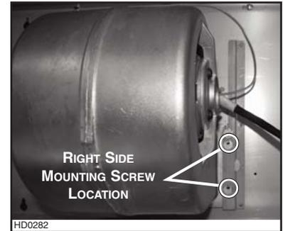
Slide the blower to disengage its flange from the retaining bracket.
