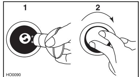
1. Install bulbs by placing the bulb leads into their grooves in the socket.
