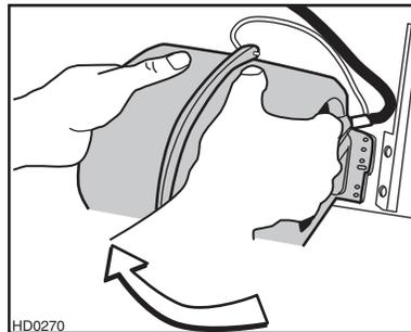
Rotate the blower and engage its flange in the back wall retaining bracket. Using a 5/16" socket and the screws previously removed, secure the blower to the hood.
