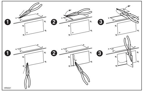
Punch out the appropriate electrical knockout hole on top (A) or back (B) of the hood. Install the wire clamp (included in parts bag).
