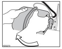
Rotate the blower and engage its flange in the back wall retaining bracket.
