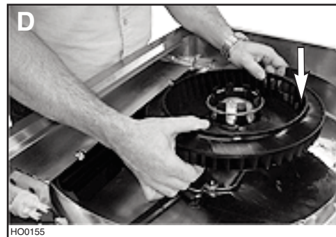
Reinstall blower wheel ensuring its tab is aligned with the yellow sticker affixed on the motor. (As illustrated below.)
