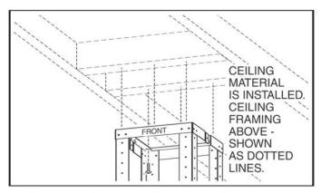
Align upper frame assembly to ceiling framing, and attach to ceiling framing with (6) 4mm x 50mm screws. Tighten securely, making sure that the upper frame bracket is tight against the ceiling.
