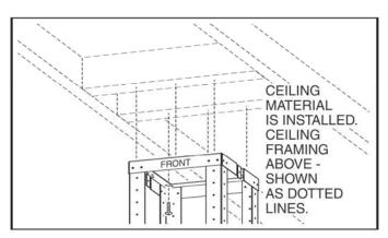
Align frame assembly to ceiling framing, and attach to ceiling framing with (6) 4mm x 50mm screws. Tighten securely, making sure that the upper frame bracket is tight against the ceiling.
