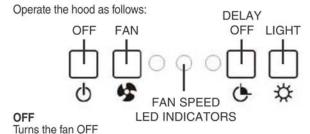
FAN (1-Pushbutton Switch, 3-Fan Speeds)
