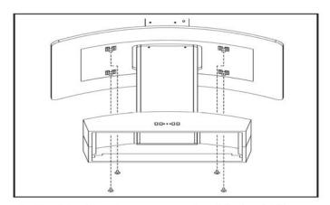
12. Carefully place glass canopy on top of the hood. Align nuts on glass canopy with holes inside the hood. Attach canopy with (4) .188" x .250" long flat head screws. Tighten screws securely but DO NOT OVERTIGHTEN.
