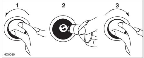
NOTE: If need be, use a rubber dishwashing glove to add grip when removing the bulb
