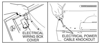
Remove <u>Electrical Wiring Box Cover</u> from inside of hood and appropriate <u>Electrical Power Cable Knockout</u> from top or back of hood.
