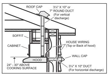
Determine whether hood will discharge vertically (3¼" x 10" or 7" Round), or horizontally (3¼" x 10" only). For vertical or horizontal discharge, run ductwork between the hood location and a roof cap or wall cap. For best results, use a minimum number of transitons and elbows.
