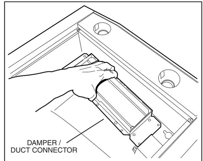
**6** Remove 2 screws holding **Damper / Duct Connector** to hood. Remove damper/duct connector from inside the hood.
