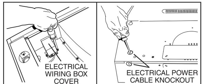
**11** Remove **Electrical Wiring Box Cover** from inside of hood and appropriate **Electrical Power Cable Knockout** from top or back of hood.
