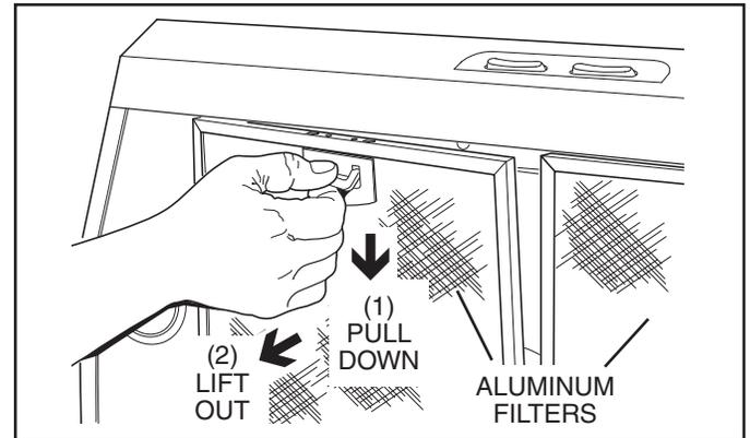
**5** Remove the **Aluminum Filters** from the hood.
