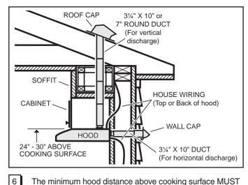
The minimum hood distance above cooking surface MUST NOT BE LESS than 24" (to top of hood).
