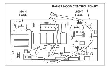
The **Range Hood Control Board** contains a **Main Fuse** and a **Light Fuse** to protect the controls from power surges. If a fuse has opened (blown), the green fan setting or light setting indicators will not operate properly when the fan or light buttons are pressed, and the fan and lights will not turn on.
