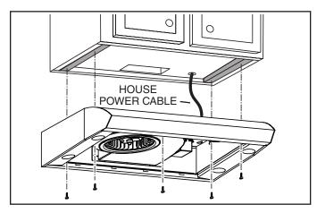
Run <u>House Power Cable</u> between service panel and hood location. Attach power cable to hood using appropriate clamp.
