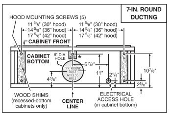
\* Note the extra wood shim and mounting screw near the cabinet front, on the cabinet center line.
