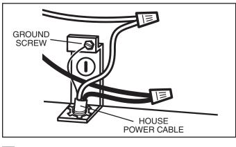
22 Connect <u>House Power Cable</u> to range hood wiring -BLACK to BLACK, WHITE to WHITE, and GREEN or BARE WIRE to <u>Ground Screw</u>. Replace electrical wiring box cover.
