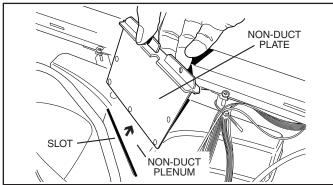
13 NON-DUCTED INSTALLATION ONLY: Remove 2 <u>Screws</u> holding <u>Non-Duct Plate</u> to <u>Non-Duct</u> <u>Plenum</u> and remove plate.
