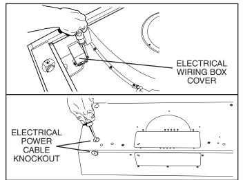
18 Remove <u>Electrical Wiring Box Cover</u> from inside of hood and appropriate <u>Electrical Power Cable</u> <u>Knockout</u> from top or back of hood.
