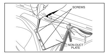
NON-DUCTED INSTALLATION ONLY: Insert short end of <u>Non-Duct Plate</u> into Non-Duct Plenum <u>Slot</u>. Attach with 2 <u>Screws</u> removed in Step 13.
