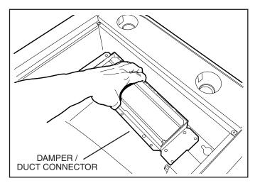
11 Remove 2 Screws holding Damper / Duct Connector to hood. Remove damper/duct connector from inside the hood.
