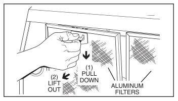
9 Remove the Aluminum Filters from the hood.
