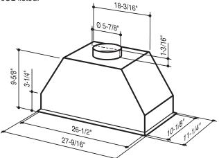
Mount power pack so bottom of unit is 24" to 30" above cooking surface.
