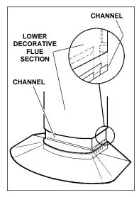
Raise upper decorative flue section and attach it to the flue mounting bracket with screws (supplied).
