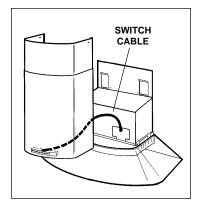
Slide the lower decorative flue section downward and into the channels on the hood.
