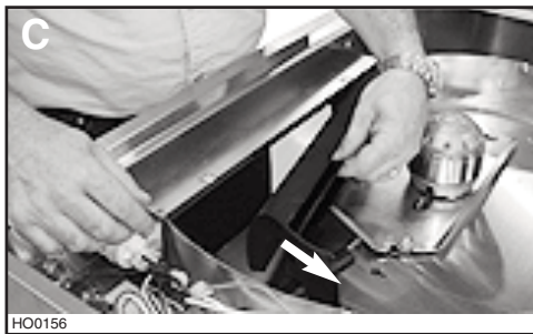
Slide the plastic deviator out and discard.
