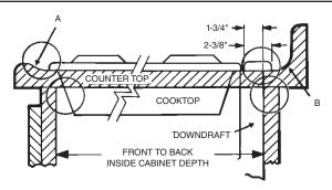
Refer to the cooktop installation instructions for dimensions of cooktop, countertop cut-out, and cabinet requirements. The RMDD3004EX can be installed in most standard 30" wide cabinets, (RMDD3604EX can be installed in most standard 36" wide cabinets), (RMDD4804EX can be installed in most standard 48" wide cabinets).
