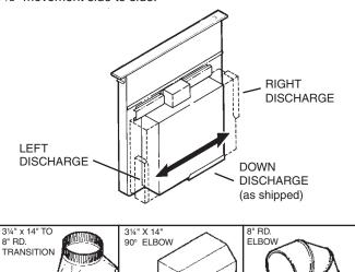
The system will operate most efficiently when the ductwork does not exceed 40 feet of equivalent duct. The chart above, shows equivalent feet of elbows and transitions. The number of feet of straight 3½" x 14" or 8" duct plus the equivalent feet of elbows or transitions to be used should equal 40 feet or less.
