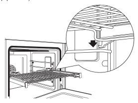
2. Slide the rack all the way in until the rear rack locks are secure on the rear rack supports and press the front rack locks onto the front rack supports.
