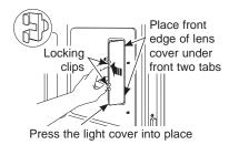
**NOTE:** If the locking clips fell from the glass lens cover, hold them on the cover, in the correct position, while replacing the cover on the light compartment.
