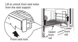
3. Firmly holding onto both the upper and lower front rack rails, pull the rack forward and remove it from the oven.
