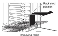
To replace a rack, place the curved end of the rack onto the rack supports. Tilt up the front of the rack and push
