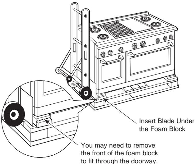
**IMPORTANT:** Do not remove the base foam block while the hand-truck is in use. Place the hand-truck blade underneath the base foam block and transport the range to the final location.
