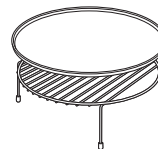
For two-level baking, place food in a metal baking dish or directly on the non-stick metal tray. Place the aluminum baking sheet or your baking dish with food on top of the wire rack. Stand the rack with food on the metal tray.
