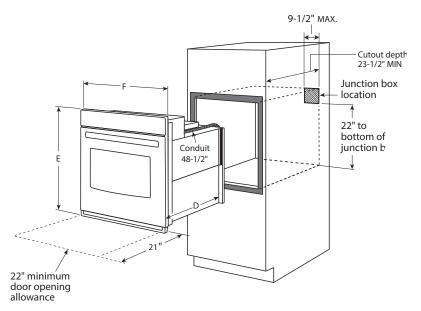
Electric wall ovens are not approved for installation with a plug and receptacle. They must be hard wired in accordance with installation instructions.
