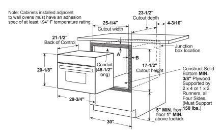
A= Allow 1" overlap of oven over bottom edge of cutout, and allow 2-3/4" overlap at top edge of cutout.
