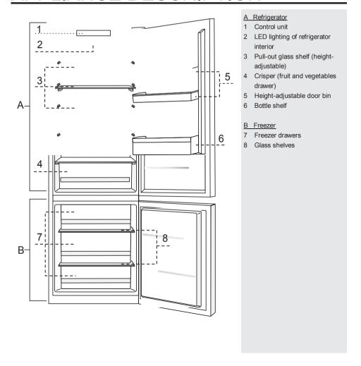
The drawers are protected against pulling out. To remove a drawer from the appliance, pull it out as far as it will go, then lift at the front and pull out completely.
