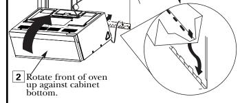
3 Insert a self-aligning screw through top center cabinet hole. Temporarily secure the oven by turning the screw at least **two full turns**after the threads have engaged. (It will be completely tightened later.) Be sure to keep power cord tight. Be careful not to pinch the cord, especially when mounting flush to bottom of cabinet.
