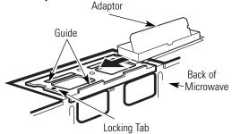
Push in securely until it is in the locking tabs. Take care to assure that the damper hinge is installed so that the damper swings freely.
