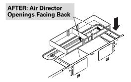
**5** Secure the blower plate to the microwave with the original screw.
