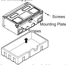
**5** Remove the screws from each end of the mounting plate. This plate will be used as the rear wall template and for mounting. Reinstall the screws into the holes where they were removed.
