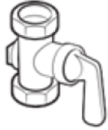
Gas line shut-off valve
