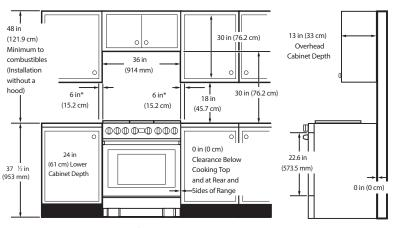
$<sup>\</sup>ensuremath{^*}$  Side clearance above cooking surface to any objects, i.e., wall.
