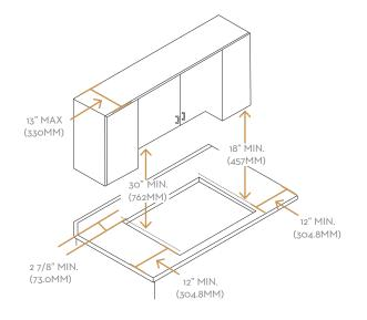
NOTE: All horizontal clearances must be maintained for a minimum of 18" (457mm) above the cooking surface.
