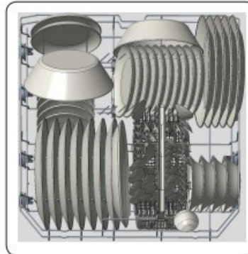
Lower rack load pattern for 10 place settings.
