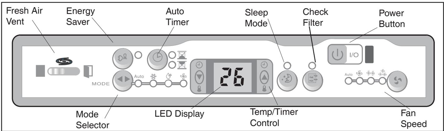
**LED DISPLAY:** Displays the following information independently; Set Temperature, Ambient Room Temperature and Auto Timer On/Off settings.
