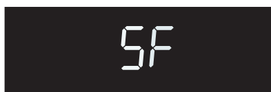
Figure 28: Display showing Sabbath failure
