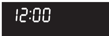
Fig. 7 12:00 displayed flashing when oven is powered up or power is restored after an interruption
