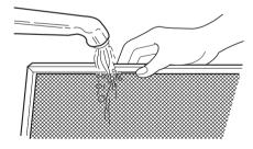
2. Soak the ventilation filters in hot water using a mild detergent. Rinse well and shake to dry, or wash ventilation filters in dishwasher. It is best to place in upper rack of dishwasher for cleaning.
