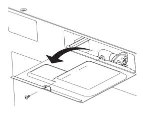
2. Remove burnt out light bulb and replace only with an equivalent 40 watt bulb available from parts distributor. Bulbs are also available at most hardware stores or lighting centers.
