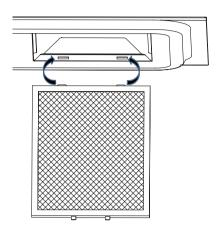
3. To reinstall the exhaust ventilation filter, infix the hooks into the holes of base plate, then pull the lever and toward oven to lock Reinstall the 2nd filter using the same procedure
