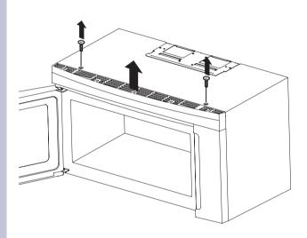
4.Remove the charcoal filter by pushing it inwards, then turn and pull it away from the unit.
