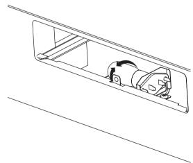
Note: DO NOT USE BULB LARGER THAN 40WATTS.
