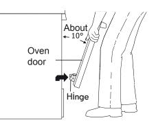
Figure 3 - Holding door for removal
