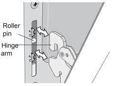
Figure 4 - Location of hinge arm and roller pin
