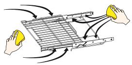
3. Shake graphite lubrication very well before applying. Apply to loading guides, and rotation pin. Repeat on both sides of the glide rack.
