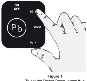
To set the Power Boost, press **hi** + when the zone is first turned on.
