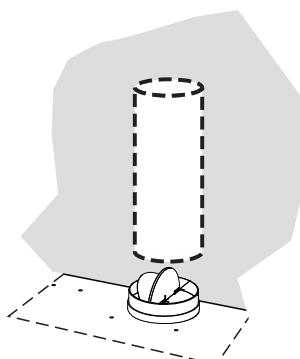
Install Roof or Wall Cap
