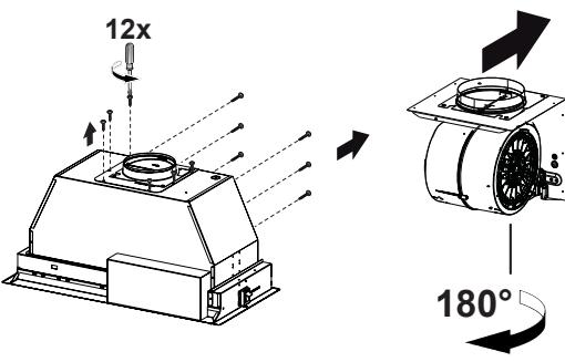
For a horizontal ducting installation the motor needs to be unsecured by first removing the 12 screws as shown.
