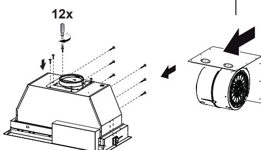
Once the screws are removed, extract the blower from the body of the Insert Hood and position it so the transition opening is facing to the rear wall (from the back remove and rotate 180 degrees to the left, and then flip it back 90 degrees as shown in the diagram).
