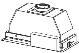
Press the charcoal filter tightly to the black grid on the blower side and rotate the filter clockwise (towards the front of the insert hood) until it locks into place. Turn counterclockwise (towards the back of the insert hood) to remove.
