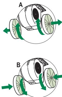
**Caution:** "When used in recirculation mode, to Reduce the Risk of Fire and Shock use only conversion kit Model FILTER 1 or FILTER1LL"
