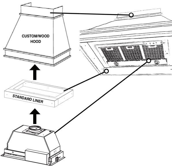
1. The custom/wood hood must have a sturdy base (3/4" plywood recommended) to accomodate the cut-out for the Inca HC. The base must be recessed to accomodate the height of the Liner (see **LINER DIMENSIONS** on Page 13). The Liner attaches to the bottom of the base using screws appropriate for the size and material of your custom/ wood hood. The Inca HC inserts into the cut-out in the Liner and base.
