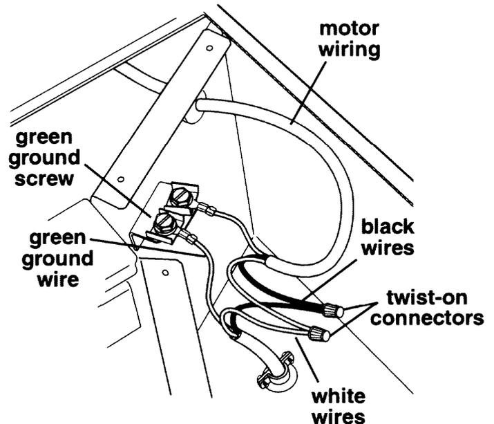
4. Replace the wiring box cover and screws taking care not to pinch the wiring under the wiring box cover.
