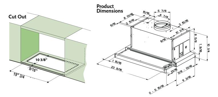
Note - When replacing the front stainless steel panel with your own custom panel, the dimensions are: 23 9/16" wide x 1 15/32" high x 13/16" deep
