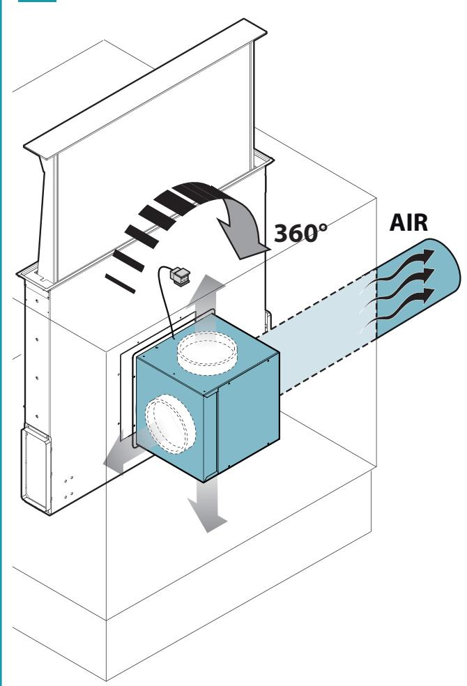
EN - Configuration with remote motor: Rectangular pipes (13); round pipes (14).
