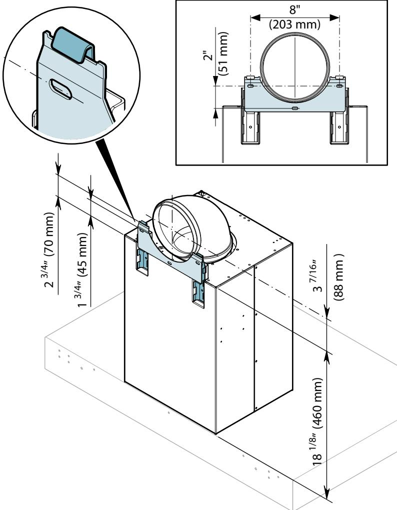
EN - Measurements for installation.
