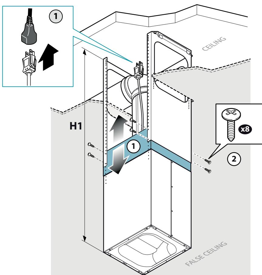
**EN** - Low ceiling installation. Securing of the bottom trestle and the motor chamber to the ceiling(14) NRS pipe installation (15).
