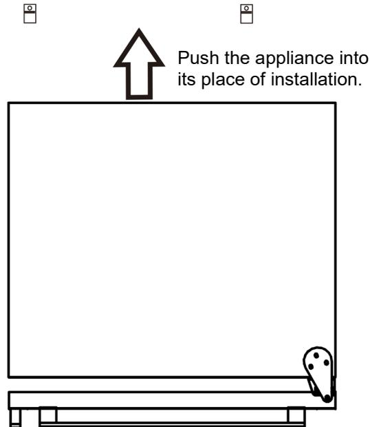
D. If the unit is not stable, pull out the appliance and repeat the previous step until the unit is stable.
