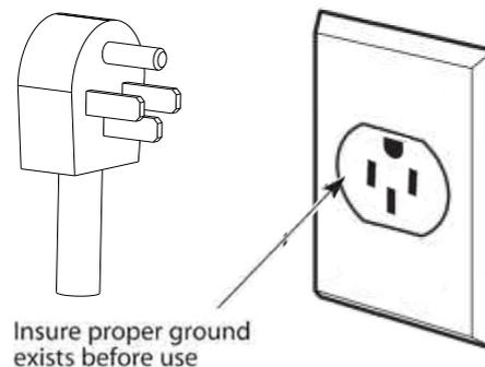
**Important: Before any operation of cleaning and maintenance disconnect the appliance from the electrical supply.**
