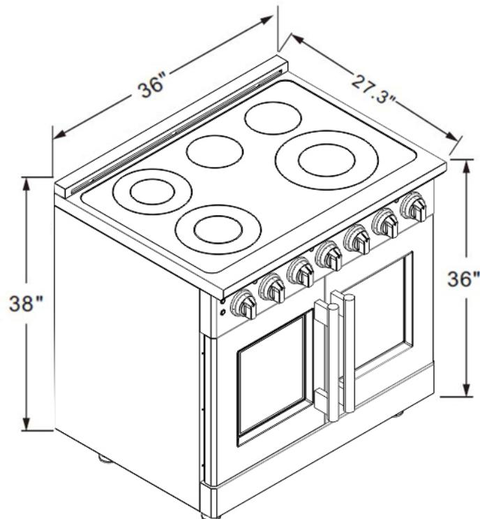
This range may be installed directly adjacent to existing countertop-height cabinets (36" or 91.5 cm from the floor). To achieve the best look, the cooktop should be level with the cabinet countertop. This can be accomplished by raising the unit using the adjustment spindles on the legs.
