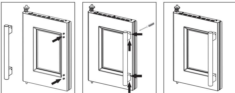
1.Align the handle with the screw on the door.
