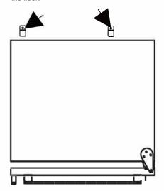
c. Push the appliance into its place of installation.
