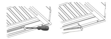
Step 1: Using the appropriate tools, remove the LED light from its slot.
