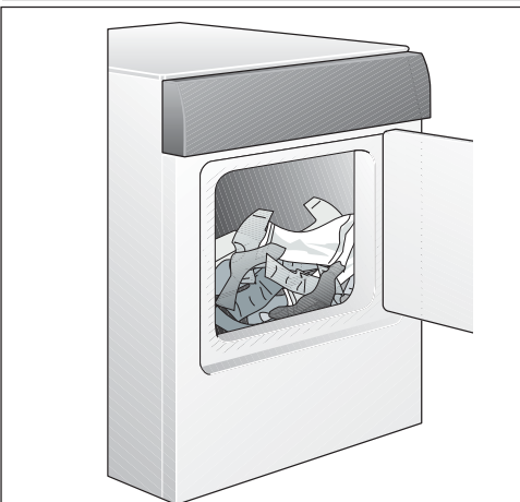
Fill dryer drum 1/3 to 1/2 full.
