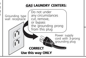
A WARNING Avoid fire hazard or electrical shock. Do not use an adaptor plug or extension cord or remove grounding prong from electrical power cord. Failure to follow this warning can cause serious injury, fire or death.
