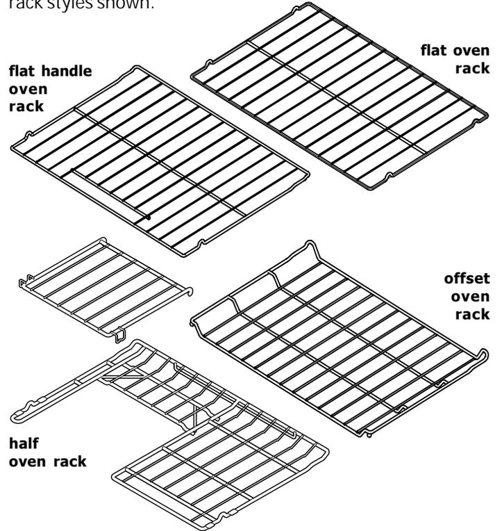
The **flat oven rack** (some models) may be used for most cooking needs and may be placed in most rack positions.
