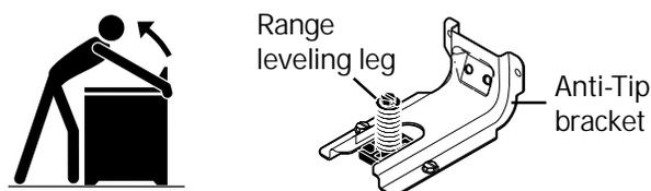
To check if the anti-tip bracket is installed properly, use both arms and grasp the rear edge of range back. Carefully attempt to tilt range forward. When properly installed, the range should not tilt forward.
