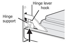
Lock engaged for door removal **Figure 1**
