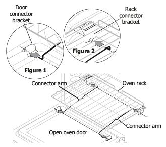
Figure 3 - Assembly of the Effortless™oven rack
