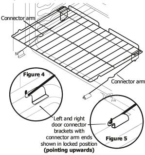
**Figure 6** - Effortless $^{\text{TM}}$  oven rack after assembly
