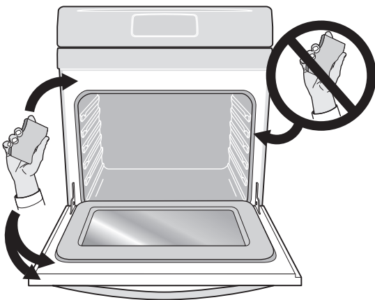
Figure 21: Clean around the oven door gasket
