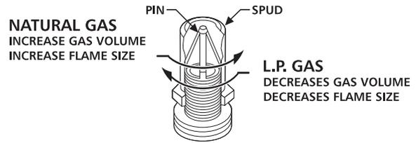
For LP/Propane to Natural conversion, loosen spuds counterclockwise (approximately 2-1/2 turns). This increases the flow of gas around the metering pin.
