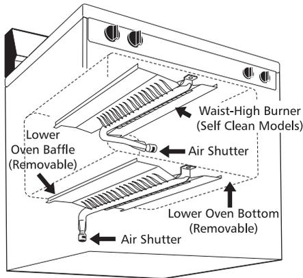
oven front frame, and pull the oven bottom out of the oven. Remove burner baffle so that the burner flame can be observed. If the flame is yellow in color, increase air shutter opening size.
