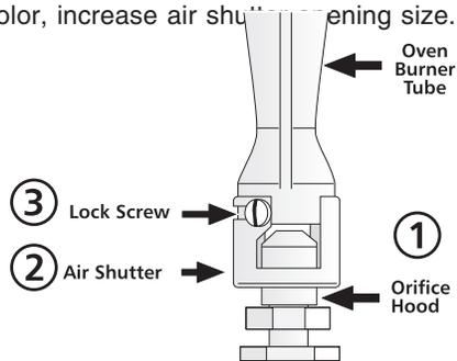
illustration below), reposition air shutter, and tighten lock screw. Replace oven bottom.
