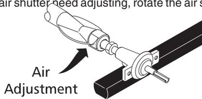
more or less air into the burner tubes as needed.
