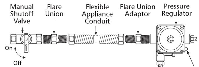
Service Shut-Off Valve Electric Ignition models only
