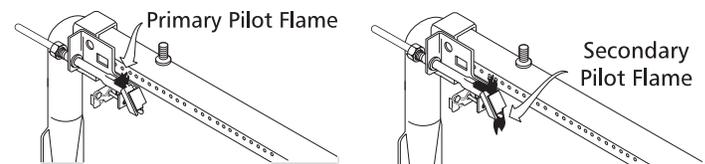
be larger with the flame extending down the slanted ramp and burning against a small metal bulb.
