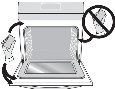
Figure 20: Clean around the oven door gasket
