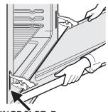
HINGE SLOT -Door removed from the range
