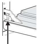
Lock engaged for door removal
