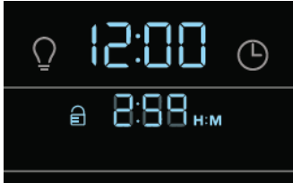
Figure 35: Clean cycle in progress
