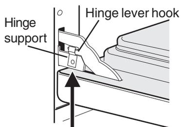
Lock engaged for door removal
