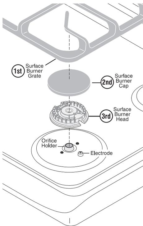
**To Remove and Replace the Surface Burner Caps and Burner Heads-** Remove in the following order: (1st) surface Burner Grates, (2nd) Burner Caps and (3rd) Burner Heads. Reverse the procedure above to replace the surface Burner Caps, Burner Heads and Burner Grates.
