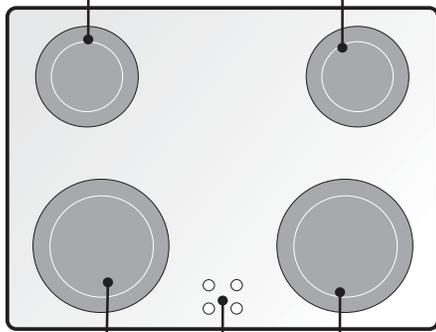
6" Single or 9" Single or 6"/9" Dual Radiant Element (Varies with models). 1 or 4 hot surface indicator lights (varies with models).
